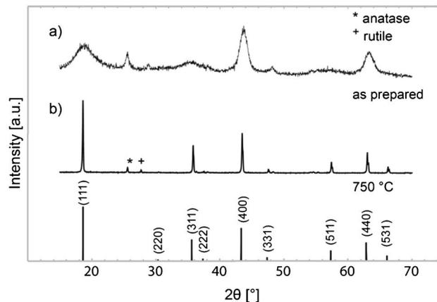
**Fig. 2** XRD scans taken with Cu-K $\alpha$  radiation of the (a) as-prepared and (b) calcined LTO, compared to reference data (ICSD 015787) (bottom). Minor rutile (+) and anatase (\*) impurities in the calcined sample are indicated by symbols above the peaks in what is otherwise a highly crystalline LTO material.
