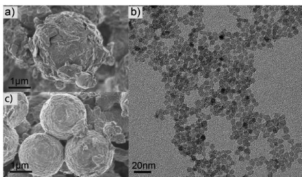
**Fig. 1** (a) SEM image of the microwave synthesis product. (b) TEM image of the material shown in (a) after ultrasonication. (c) SEM image of the LTO microspheres after calcination in air at 750 °C.
