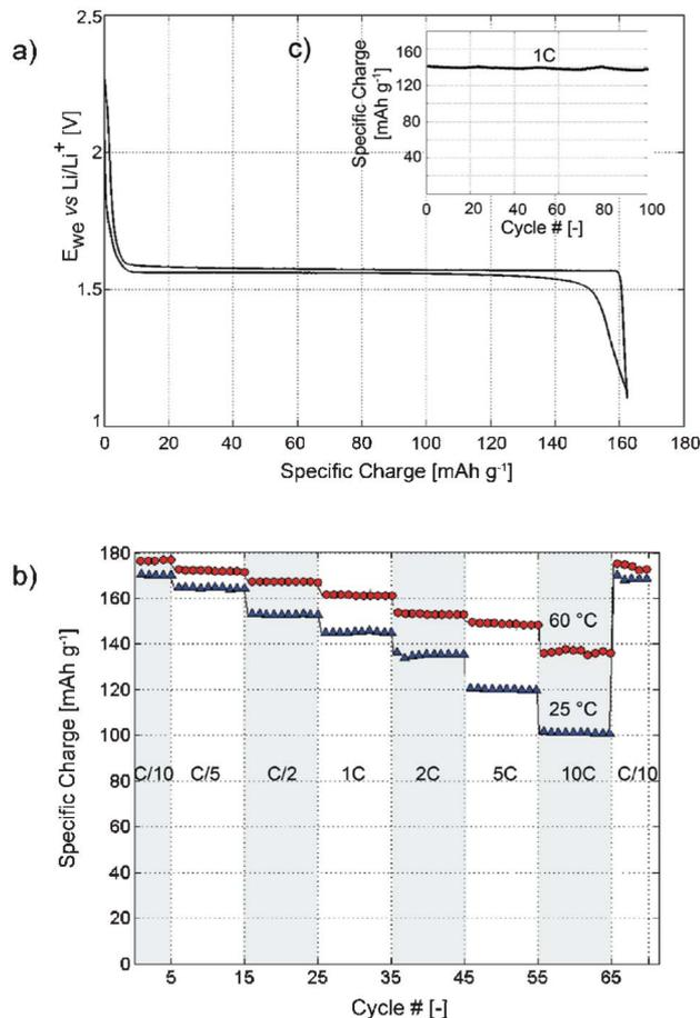
**Fig. 3** (a) Specific charge vs.  $E_{we}$  of a LTO/lithium half-cell cycled galvanostatically at 0.1 C, exhibiting a flat plateau at 1.55 V indicating reversible insertion of lithium ions. (b) Specific charge dependence of the C-rate for the same cell at room temperature (blue) and to 60 °C (red). (c) Specific charge for 100 cycles at a 1 C rate at room temperature demonstrate cycling stability.
